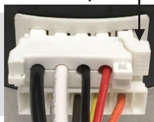
White Voltage Plug 115vac Systems
